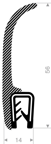
245.00.876 pvc + Sponge rubber clamping range 1-3 mm roll length 25 meter
